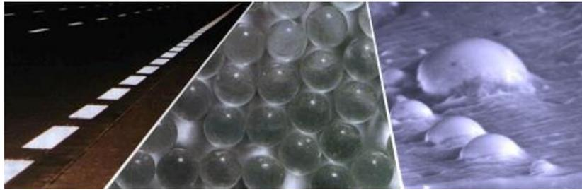
Glass beads for road markings are added, either premixed or dropped on, to add retroreflective properties to the road marking products. Without the glass beads road markings can't stand out in the dark. Glass beads are also fit for industrial applications such as surface treatment and in product engineering as additives for plastics and coatings.
